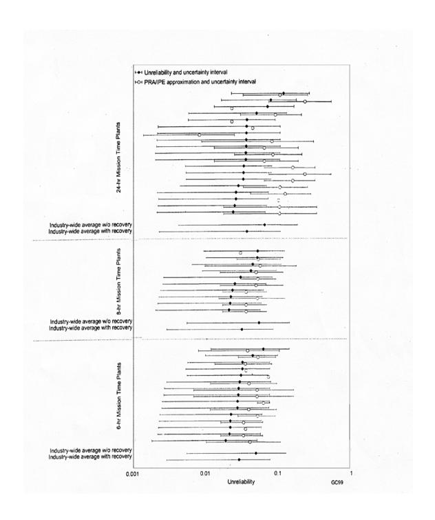
Figure 1 "Preliminary unit average emergency diesel generator unreliability compared to the unreliability estimates using the probabilistic risk assessment/ individual plant examination emergency diesel generator performance assumptions."
