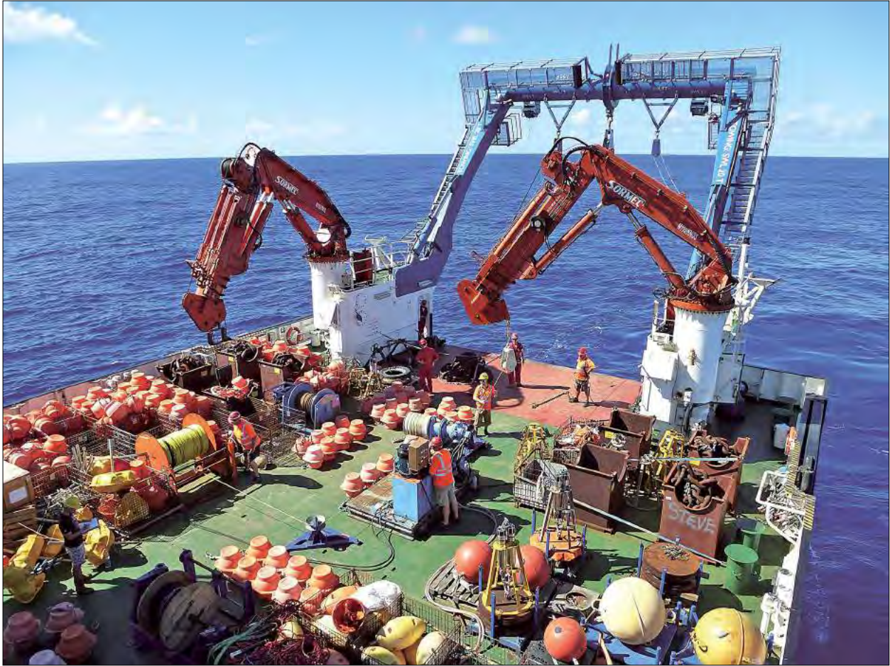
Figure 4.2.1 The aft deck of the RRS Discovery during the deployment of a deep ocean mooring that forms part of an array measuring the transport of heat northwards through the North Atlantic Ocean. November 2015. © Peter Brown, National Oceanography Centre, Southampton, UK.
