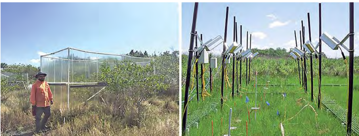
Figure 3.4.3 Two approaches to experimentally warming tidal marsh ecosystems. Left: Chambers erected on a Florida USA saltmarsh raise air temperature by 2–3°C. The chamber has negligible effects on soil temperature. Right: A brackish marsh in Maryland USA is actively heated (1.7–5.1°C) aboveground by infrared lamps and belowground by cables to a depth of 1.5 metres. © Adam Langley (left) and Roy Rich (right).
