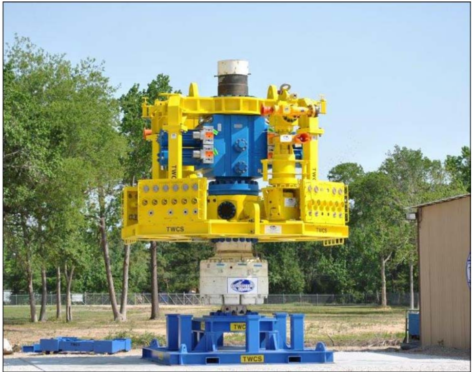
Figure 3: A Capping Stack Ready for Deployment
