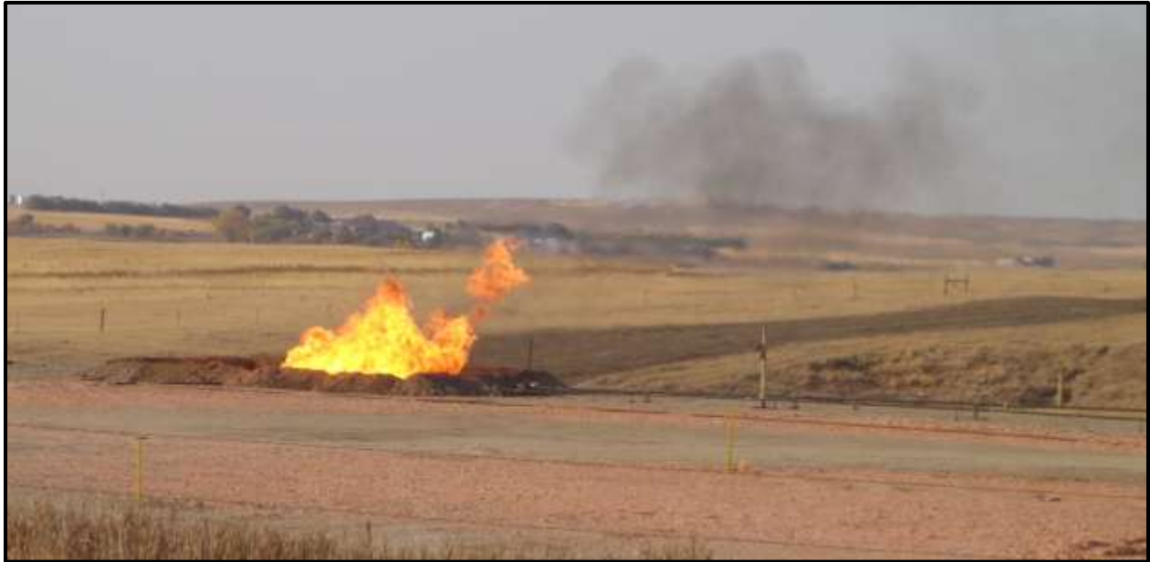
Figure 3. Flaring of natural gas and contaminates at a producing oil and gas well.
