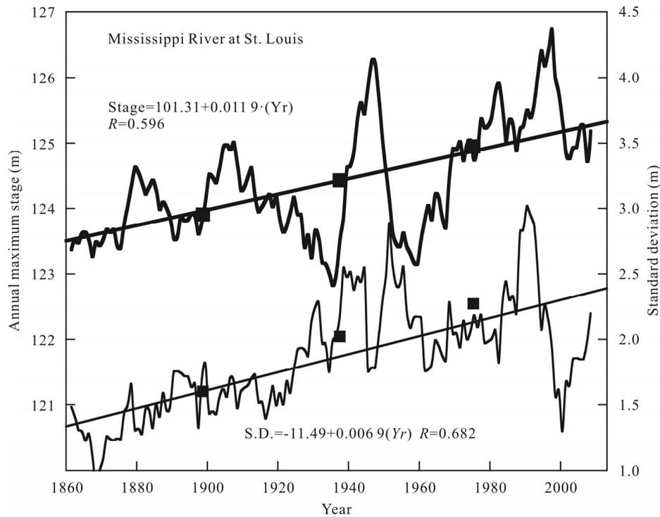
**Figure 1.** Ten-year running averages of the annual maximum stage (m rel. MSL) and the associated standard deviation, plotted vs. the mid-year of the running interval. Linear regressions are shown. Squares plotted at 1937 indicate the mean and standard deviation of the entire (1861–2013) population, while the flanking squares indicate the respective values for the first and second halves of the data.
