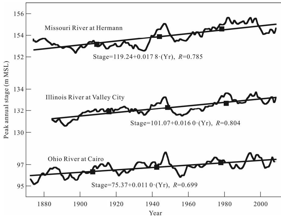
**Figure 2.** Ten-year running averages and linear regressions of the annual maximum stage (m rel. MSL) for sites along the lower Missouri, Illinois and Ohio rivers. Center squares indicate the means of each entire population, while the flanking squares indicate the respective means for the first and second halves of the data; the squares are collinear and were used to define factor  $a$  in Table 1. Mean annual flood stages increased ~2 m at all three sites over the period of record.
