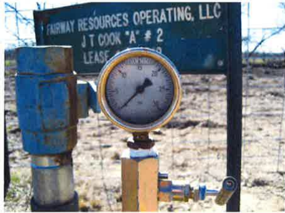
PHOTO #5993 – VIEW OF BRADENHEAD GAUGE.
