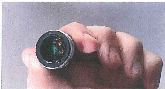
Particles observed in aerators, including the one shown here, include scale minerals released from plumbing materials, which can contain high levels of lead.
